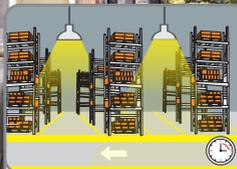
After the hold-time, the sensor dims the fitting to the pre-set low light level if no motion is detected.
