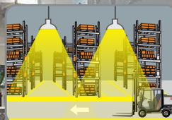
With insufficient natural light, the sensor switches on automatically when presence is detected.
