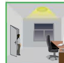
With insufficient natural light, the sensor switches on the light automatically when person enters the (options) standby level after the room. The lamp never switch off with presence, even the nature light is sufficient.
