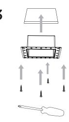
Fix to the ceiling using 6x Stainless Steel Drywall Screws
