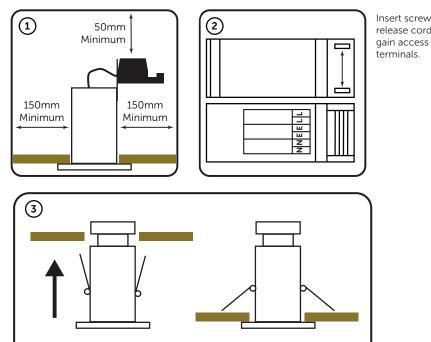
Insert screwdriver to release cord grip to gain access to tool-less
