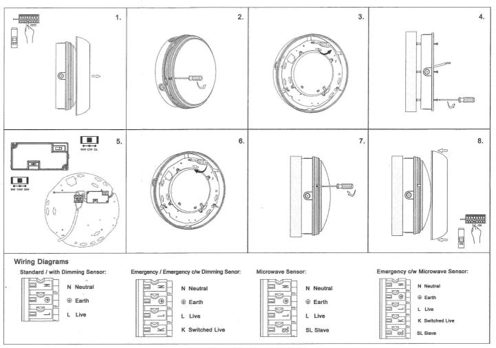
Slave function is only available in the on/off sensor versions up to a maximum of 10 additional AQUA1 fittings
