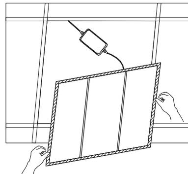
① Remove the ceiling plaster slab.
