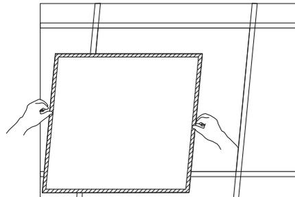
① Remove the ceiling plaster slab.
