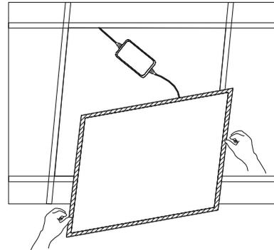
① Remove the ceiling plaster slab.
