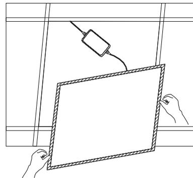
② Feed the main AC wire in driver terminal block respectively, connect the panel light and driver.
