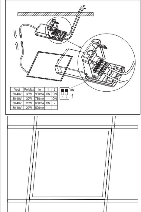
For color changeable model (controlled by Slide Switch in lamp), please select light color before installation, see below picture.
