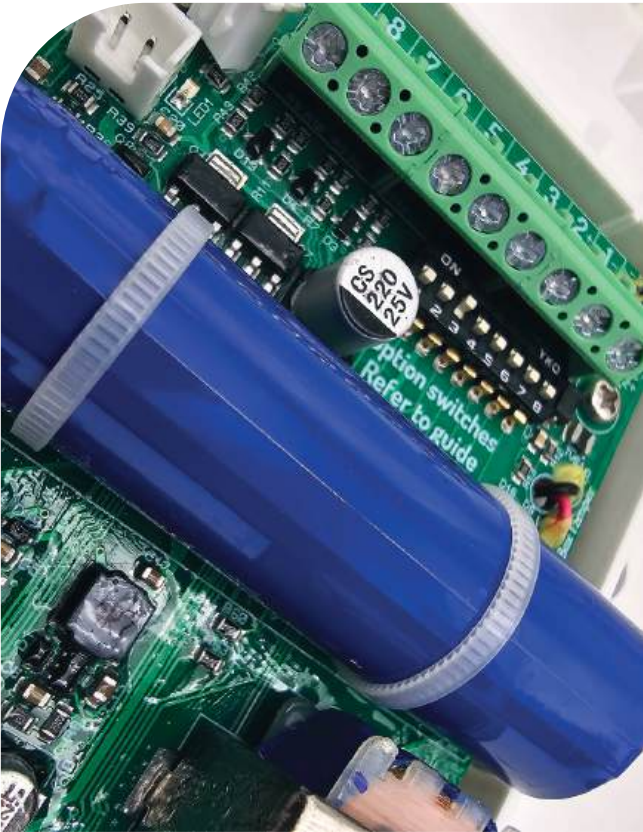
ENGINEER HOLD-OFF: During initial setup, it allows the installer to connect the backup battery without activating the sounder.
