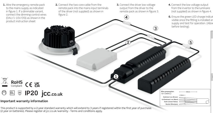
onnect the low voltage output om the invertor to the luminaire ot supplied) as shown in figure 4.
