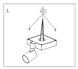
Remove the 4 screws and the spike as indicated above
