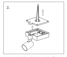
Remove the back plate and spike from the body
