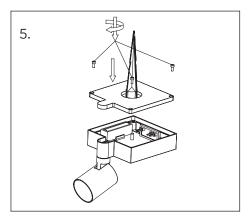
Refit theback plate onto the body and refit the 4 screws, then re-attach the spike
