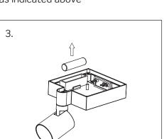
Disconnect and remove the old battery
