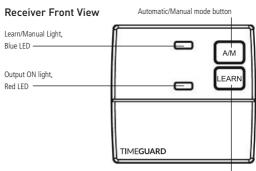
Learn button enabling communication between the transmitter and receiver, also control button for output in manual mode
