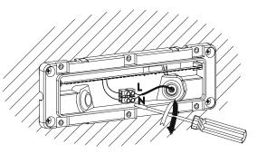
• Re-fasten the clear plastic cover using the cover fixing screws previously removed.
