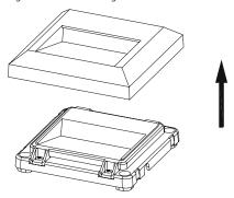
Undo the 4 cover fixing screws and remove the clear plastic cover.
