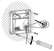
Terminate the cable into the terminal block (See section 5. Connection Diagram)
