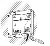
• Re-fasten the clear plastic cover using the cover fixing screws previously removed.
