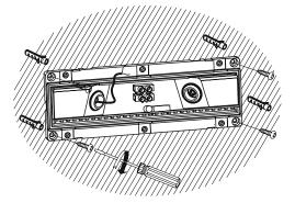
Terminate the cable into the terminal block (See section 5. Connection Diagram)
