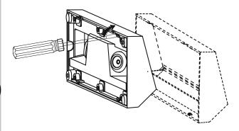
Undo the 6 cover fixing screws and remove the clear plastic cover.
