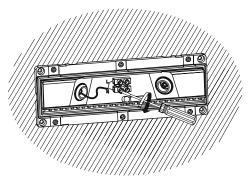
• Re-fasten the clear plastic cover using the cover fixing screws previously removed.
