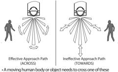
A moving human body or object needs to cross one of these zones to activate the sensor. The optimum height for this is between 1.5m - 2m mounting height. Careful positioning of the luminaire is required to ensure the best performance from the PIR and the appointed approach path.
