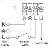
**Note:** Any floodlight connected to the L4 Switch Live terminal 'Live Output' will be controlled by the Photocell
