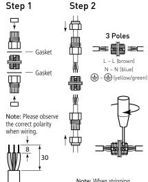
Min. cable diameter 5mm. Max. cable diameter 8mm. Note: When stripping the cables please use the measurements shown.
